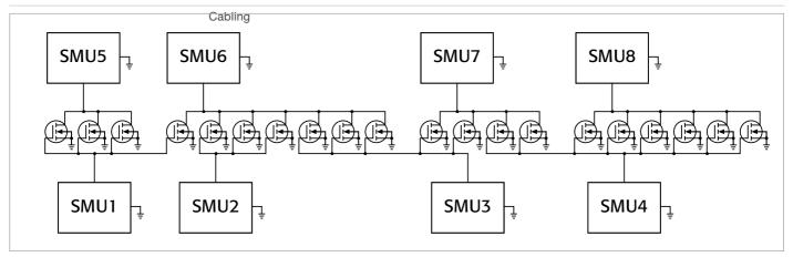
Example of using eight SMUs to stress 20 devices in parallel for HCI and NBTI. A separate ground unit (GNDU) is used for common terminals.
