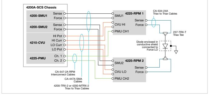
Connection diagram when using 4225-RPM Remote Preamplifer/Switch Module.
