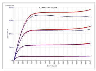
Minimize self-heating effects with ultra-fast pulsed I-V.
