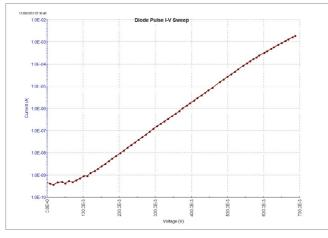
4225-RPM provides lower current ranges for pulse applications.
