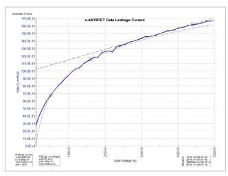
Sub-fA measurements with optional 4200-PA preamplifier module.
